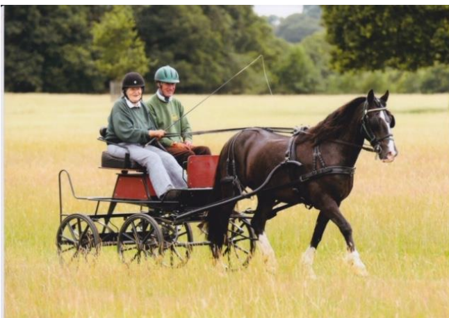
A typical carriage used for countryside access, 1.5metres wide approx. and approx. 200kg in weight (without horse & driver) caption and photos supplied by BHS
